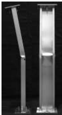
(a) Local buckling
