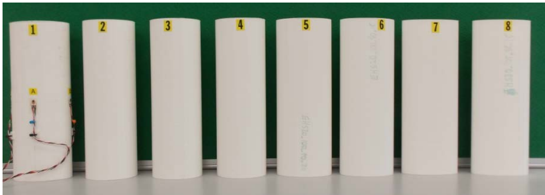
Figure 2: Fabricated EHS stub specimens.
