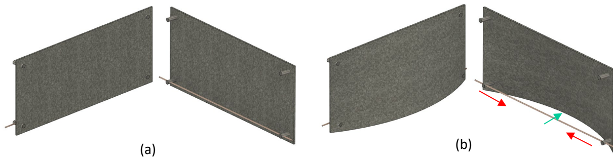
Fig. 2. The proposed ventilation panel by Formentini and Lenci, 2018 in (a) closed and (b) open positions. NiTi SMA wires connected to the plate to stress the plate into the buckled position
