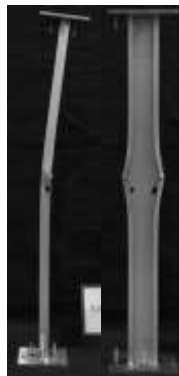
(b) Distortional buckling
